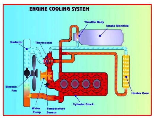
The pump draws the coolant/water from the bottom of the radiator, forcing it through the water jackets and passages, and ejects it into the upper radiator tank. The coolant then passes through a set of tubes to the bottom of the radiator from which the cooling cycle begins.
