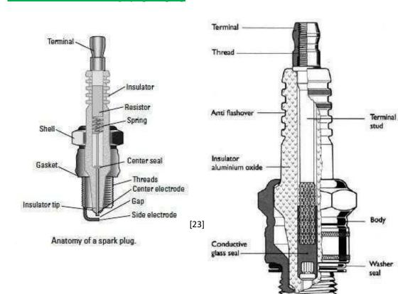
A typical spark plug used in case of petrol engines. It is shown in the figure. It mainly consists of a central electrode and ground electrode. Central electrode is covered by means of porcelain insulating material. Through the metal screw the spark plug is fitted in the cylinder head plug.
