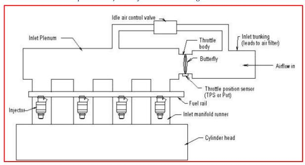
Multi-point fuel injection (MPFI) injects fuel into the intake port just upstream of the cylinder's intake valve, rather than at a central point within an intake manifold. In MPF systems fuel is injected to the cylinders in groups in which fuel is injected at the same timetoall the cylinders
