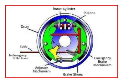
The drum brake has a metal brake drum that encloses the brake assembly at each wheel. Two curved brake shoes expand outward to slow or stop the drum which rotates with the wheel.
