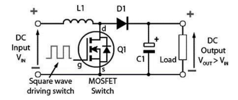
If the switch is kept as low (off), it discharges the energy. Here, the output of the capacitor is assumed as high that is sufficient for the time constant of an RC circuit on the output side. The huge time constant is compared with the switching period and made sure that the steady-state is a constant output voltage. It should be Vo(t) = Vo(constant) and present at the load terminal.
