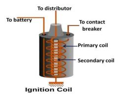
Ignition coil is the source of the high voltage pulses of current in the ignition system. The coil stores the energy in the magnetic field around the primary winding and at the required instant of ignition, transforms it into a pulse of high voltage current in the secondary winding. From here it is delivered to the correct spark plug via the high tension (HT) cables and distributor.
