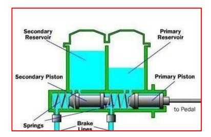
When we press the brake pedal, it pushes on primary piston of master cylinder through a linkage. Pressure is built in the cylinder and the lines as the brake pedal is depressed further. The pressure between the primary and secondary piston forces the secondary piston to compress the fluid in its circuit. If the brakes are operating properly, the pressure will be same in both the circuits. If there is a leak in one of the circuits, that circuit will not be able to maintain pressure.
